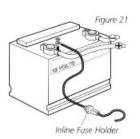
fuse in the connection. If you must wire the control head directly to a battery, be sure to install an inline fuse holder
